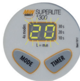
Timer flashes low battery 5-10% charge!
